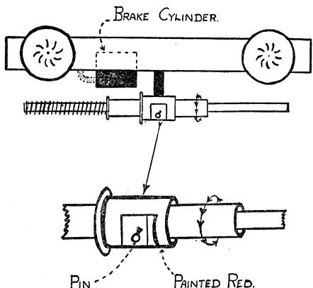
The pin must be replaced after this has been done, and the cylinder rendered inoperative in accordance with clause II of the general regulations for working the vacuum brake. The train must then stop at the next point where a C. & W. examiner is on duty, and he must be told what has been done. Under no circumstances must any attempt be made to release the brake by levering the brake arms as this may cause serious damage.
