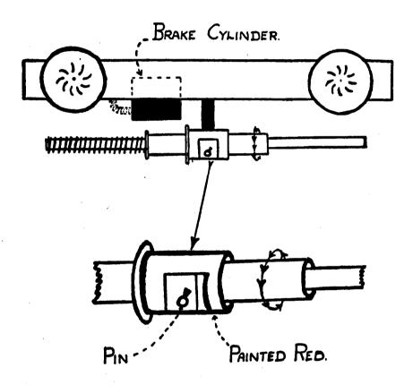
The pin must be replaced after this has been done and the cylinder rendered inoperative in accordance with clause 11 of the general regulations for working the vacuum brake. The train must then stop at the next point where a C.&W. examiner is on duty and he must be told what has been done. Under no circumstances must any attempt be made to release the brake by levering the brake arms as this may cause serious damage.
