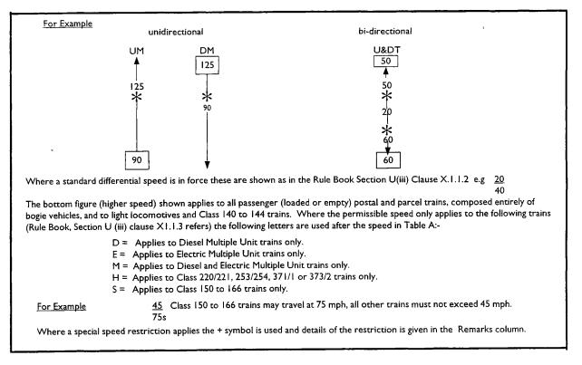
On single lines and bi-directional where different speeds apply for each direction the speeds will be shown adjacent to the line together with an arrow head indicating the direction in which they apply:-
