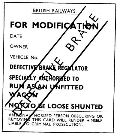
Although these labels are marked 'Defective Brake' the provisions of Rule 170 Clause (b) are modified in respect of the vehicle to which the labels are attached in that it may be loaded and run in traffic as an unfitted or piped vehicle.
